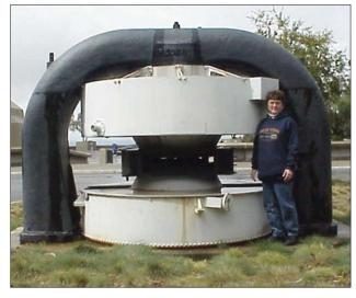
ABOVE: Figure 10. The magnet used for the 27-inch cyclotron (operational 1932), then modified to the 37-inch cyclotron (operational five years later), is now standing outside the Lawrence Hall of Science. The magnet, originally built for power communication between the U.S. and Europe in World War I, was acquired by Lawrence as war surplus.
